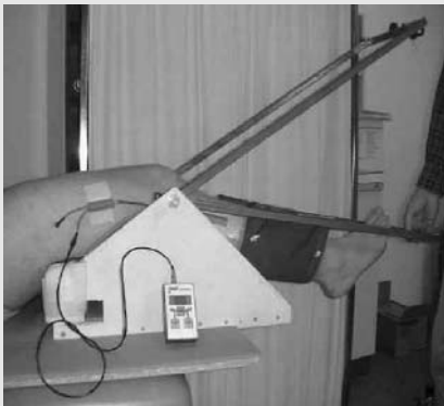
Fig. 3 ▲ Testing apparatus with goniometer for passive angle reproduction test
